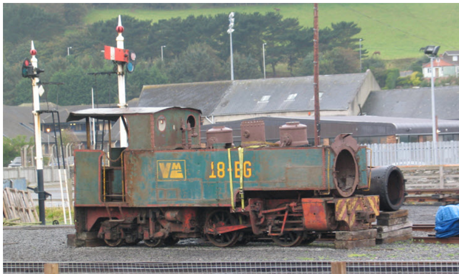
One of the engines currently at Aberystwyth, W.G. Bagnall's 1928 0-4-4T OC 2 ft (610 mm) 18BG, ex Sha Tau Kok Railway and Victorias Milling Co., Negros Occidental. Photo to Denis Bates.
