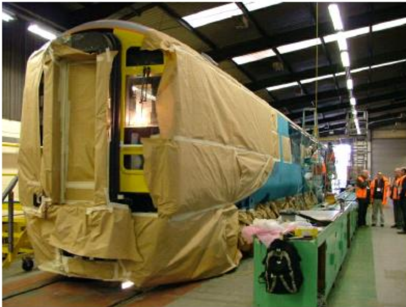
Unit 158840 at LNWR, Crewe during the refurbishment. The unit is partially masked off for the application of the darker paint coat.
