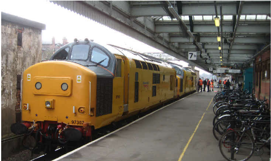
Converted Class 37's 97301 & 97002 at Shrewsbury 1st April. Designed to pilot special trains and haul infrastructure trains using ERTMS equipment. Not seen on Cambrian yet.
